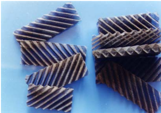
Figure 5. Corrugated gauze of metal.
