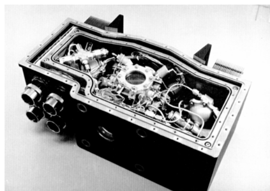
Figure 3. BDPU TC3: Experimental equipment for bubble growth and condensation study on board Spacelab
